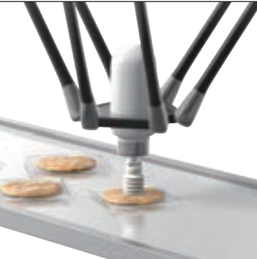
Adsorption conveyance of foods
