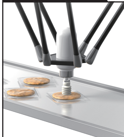
Adsorption conveyance of foods
