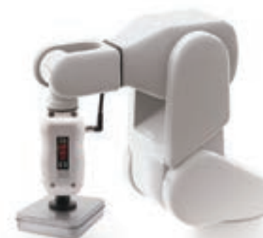
SGE series electric suction hand (e-HAND)
